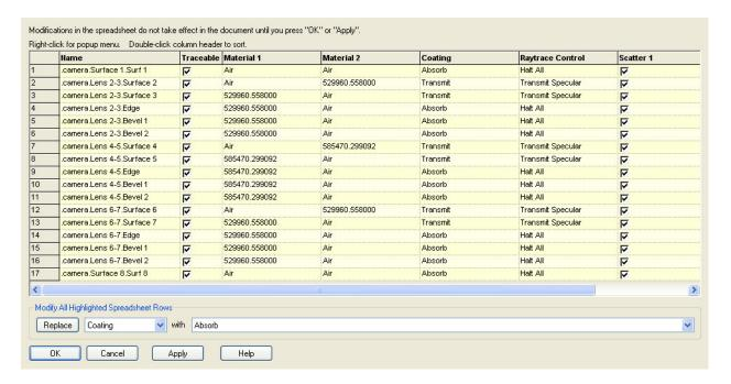
We are going to use this interface to replace all of our Transmitting surfaces with the default "Standard Coating", which allows 96% power transmitted and 4% power reflected, and the default "Allow All" raytrace control, which allows rays to be split into reflected and transmitted components at an interface. While holding down the "Ctrl" key on your keyboard, select the rows in the spreadsheet which have the "Transmit" coating.
