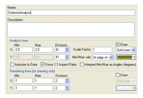
After completing the specifications above, hit the OK button to create the new analysis surface. We can assign this analysis surface to our detector by expanding out the Analysis Surface(s) folder and our geometry tree (so that we can see "Surf 8") and then dragging and dropping the DetectorAnalysis node onto Surf 8.
