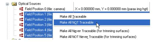
When tracing incoherent sources it is generally a good idea to remove any "grid-ness" of the source definition. Double click on the Field Position 0 source to open its dialog and
