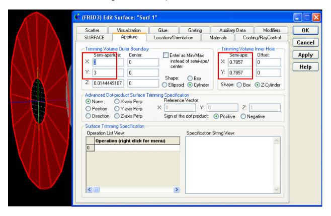
Now that we have an annulus surface, we need to make it optically relevant. On the Coating/RayControl tab of the surface dialog, apply the Absorb coating and the Halt All raytrace control.
