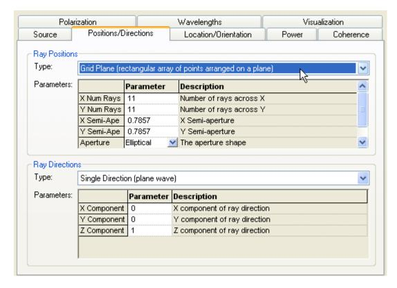
With incoherent sources, having grid positions and directions specifications can cause aliasing artifacts in the calculated energy distributions (source grid overlapping with an analysis grid). To remove the potential of this occurring, we change the ray positions type from Grid Plane to "Random Plane" while maintaining the same aperture size and shape.
